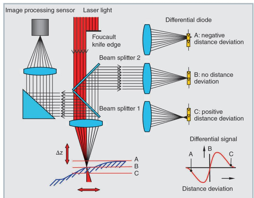
Figure 1: Laser sensor using the Foucault principle integrated into an image processing sensor (illumination systems not shown) (© Werth)
