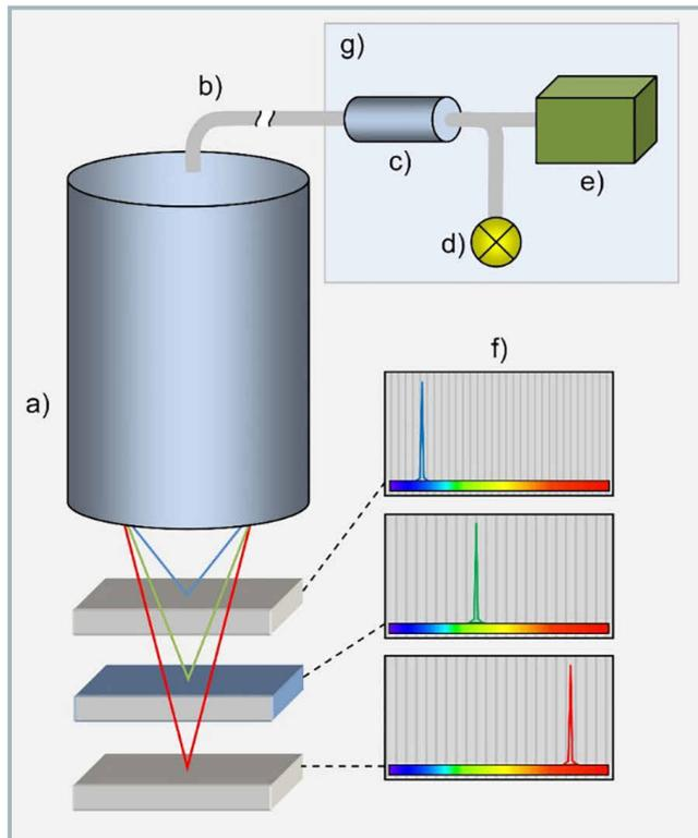
cal area sensors, in contrast to focus variation sensors, can also measure reflecting surfaces, for example, regardless of the contrast of the workpiece surfaces. Applications include the measurement of stamping tools or coin embossing punches. ■
