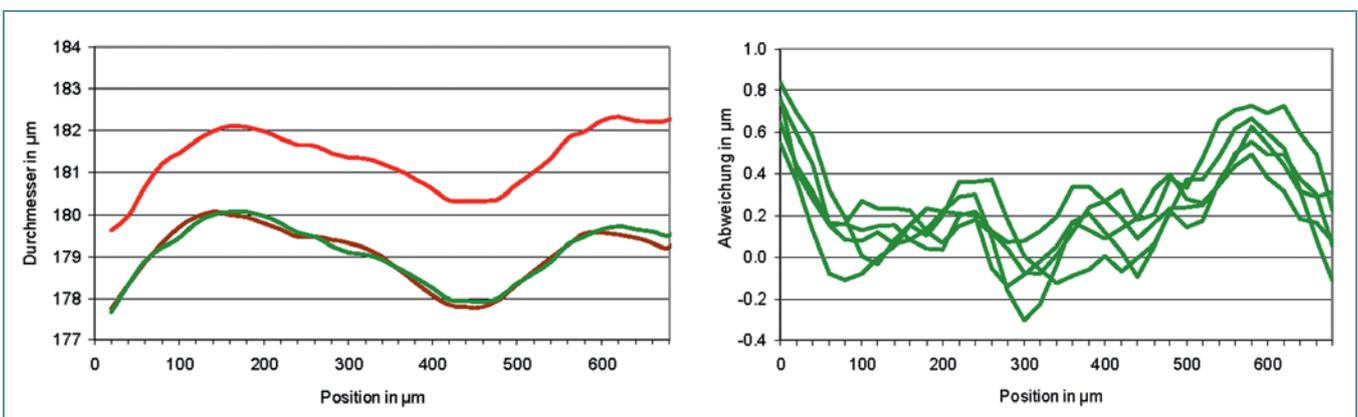
Figure 7. After correcting the CT measurement of the diameter (curve along the injection hole) of a diesel injection nozzle (left, red) by means of a reference measurement with the Werth Fiber Probe (left, brown) the measuring deviations of several corrected CT measurements (right) stay below one micron.
