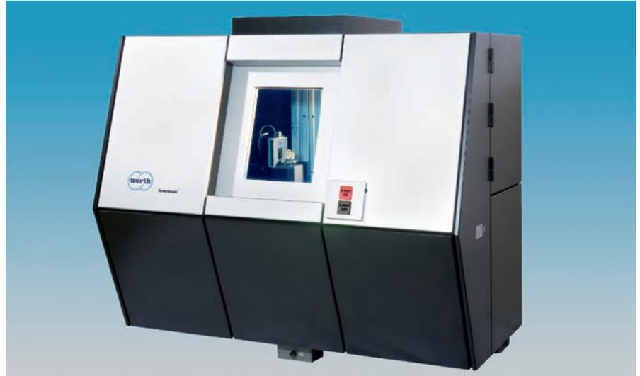
Figure 1. Coordinate measuring machine with computer tomography for complete and precise measurements, even for workpieces that are difficult to penetrate radiographically.
