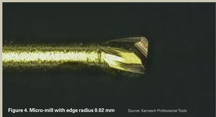
**Figure 4. Micro-mill with edge radius 0.02 mm**
