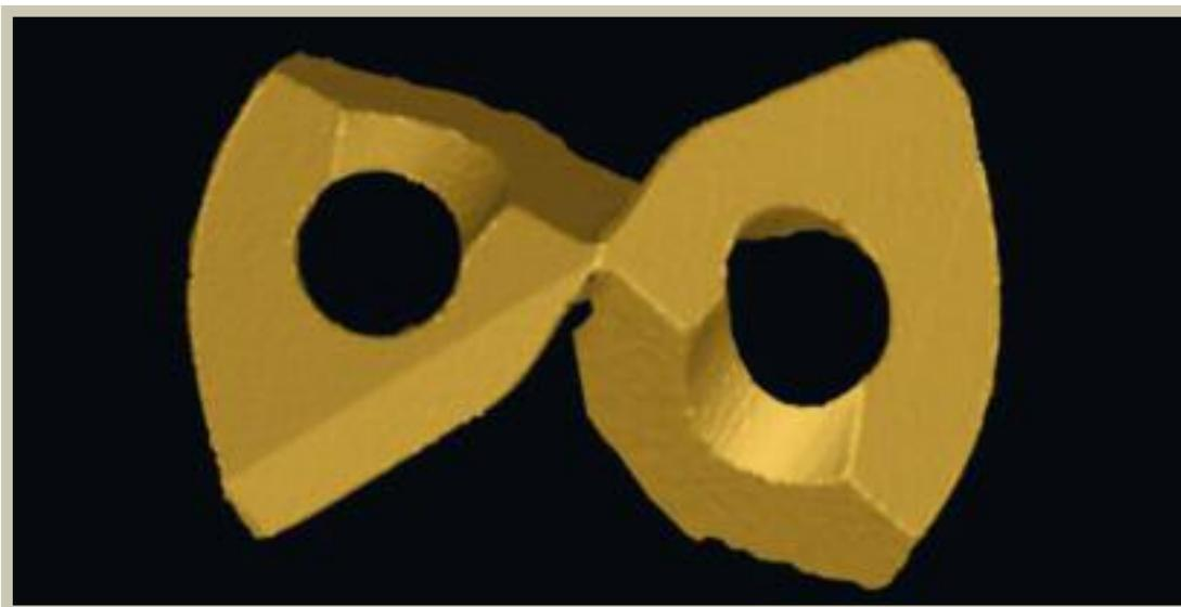
**Figure 6. Result of a CFL measurement on a micro-drill tip: STL with high detail resolution**
