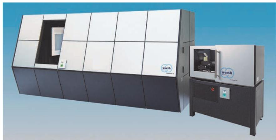
Figure 2. Modern machines with X-ray tomography sensors enable workpieces of various sizes and tolerance classes to be measured during production. Left: CT machine for measuring large workpieces with X-ray voltages up to 450 kV; right: compact, low-maintenance measuring machine with 160 kV X-ray for smaller plastic and metal components (© Werth Messtechnik)
