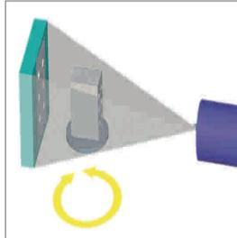
*The measured object is rotated 360° for complete X-ray capture*
