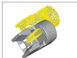
*Automatic rough alignment of the point cloud to the CAD model*
