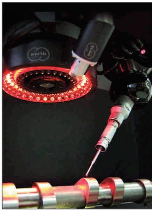
Due to the complexity of many measuring tasks the use of several sensors on the same sample is required often.
