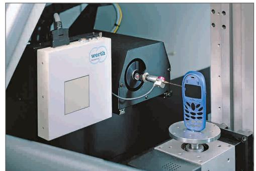
*Precise and Fast with Tomography – Thanks to Werth Multisensors*
