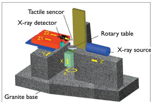
*Mechanical construction of the Werth TomoScope®*
