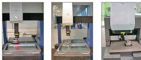
*A measurement station was integrated in the production line in each processing area with a multisensor coordinate measuring machine configured for the measurement tasks.*
