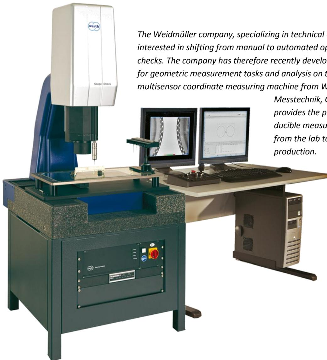
*The Weidmüller company, specializing in technical connectors, is interested in shifting from manual to automated operator self-checks. The company has therefore recently developed a standard for geometric measurement tasks and analysis on the basis of a 3D multisensor coordinate measuring machine from Werth*
