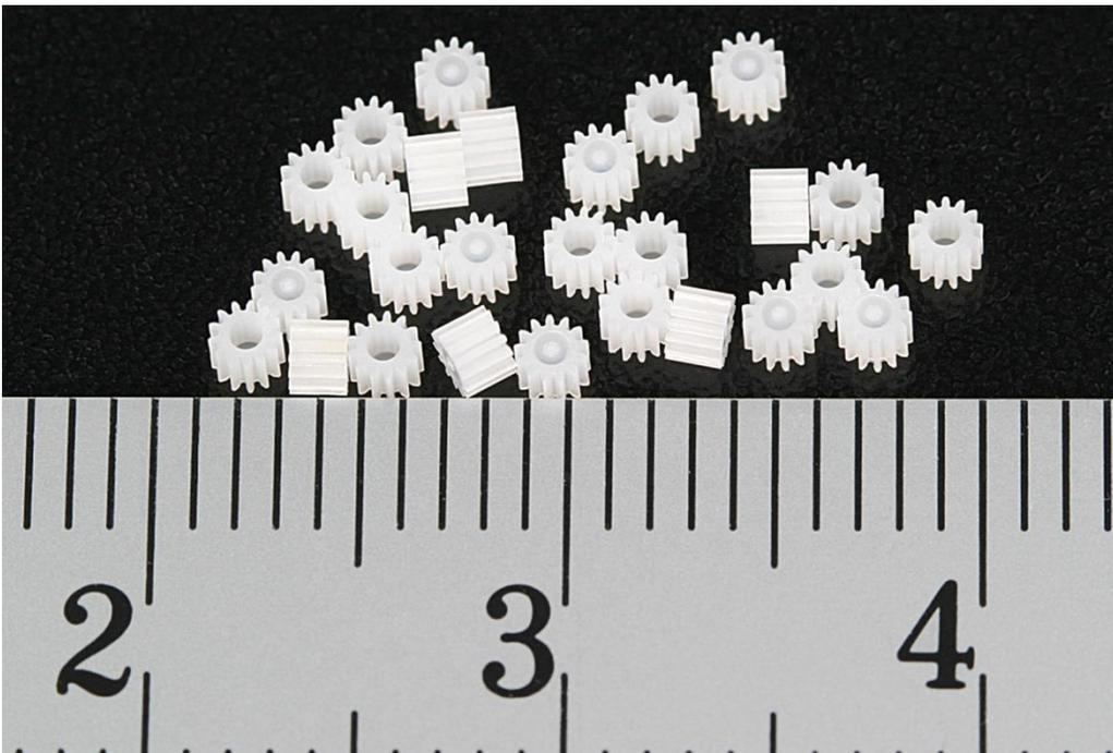
*Tiny planetary gears like this are found in the GP6 planetary gearbox. Measuring them is a challenge: gears with module 0.12 (tip diameter 1.908 mm, root diameter 1.347 mm, number of teeth 13, material Delrin 100; image: maxon motor).*
