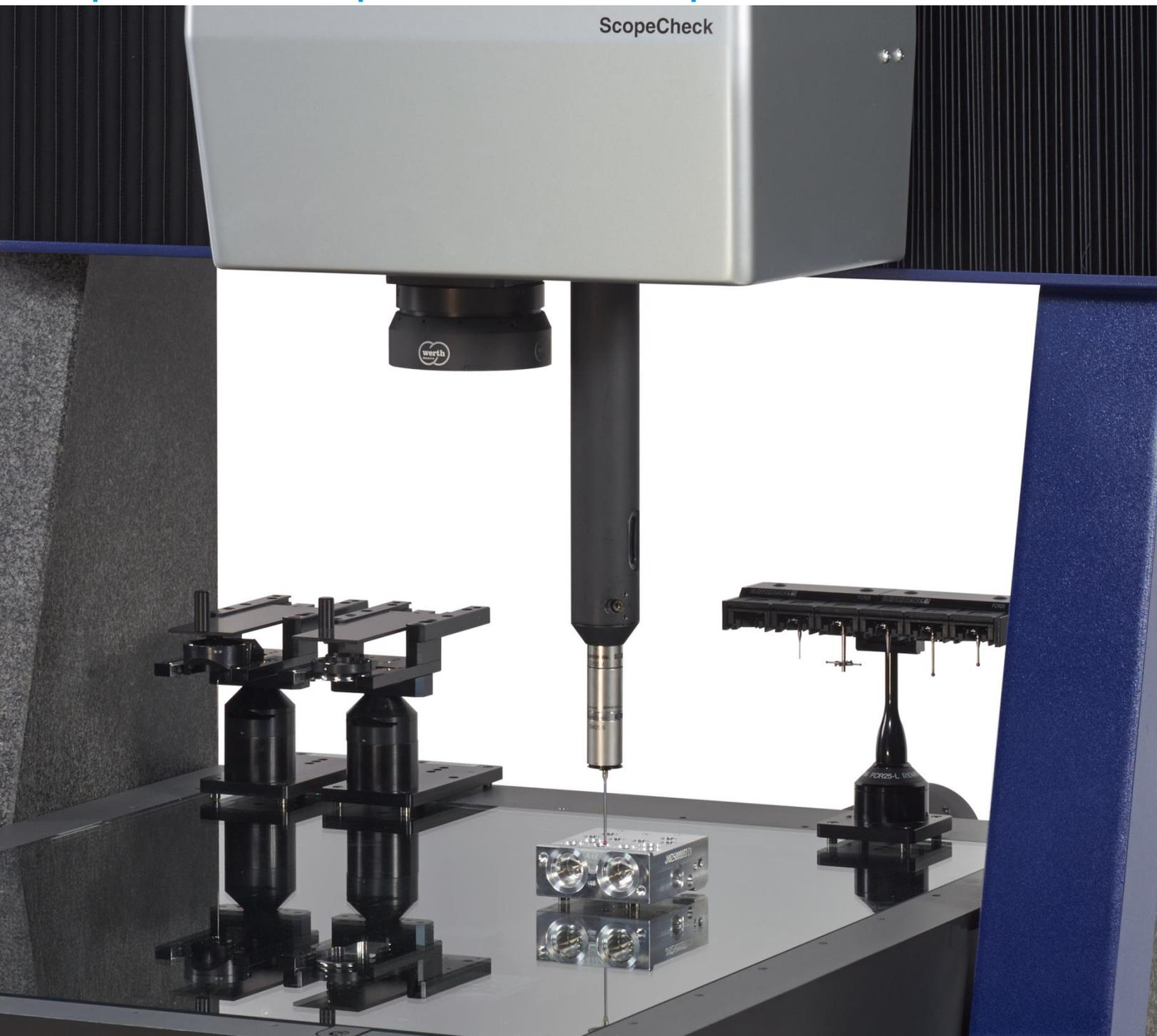
*ScopeCheck® FB DZ – collision-free measurements also on the shop floor: dual ram approach for optimal measuring with each sensor, for example image processing sensor or touch probe (cover picture)*
