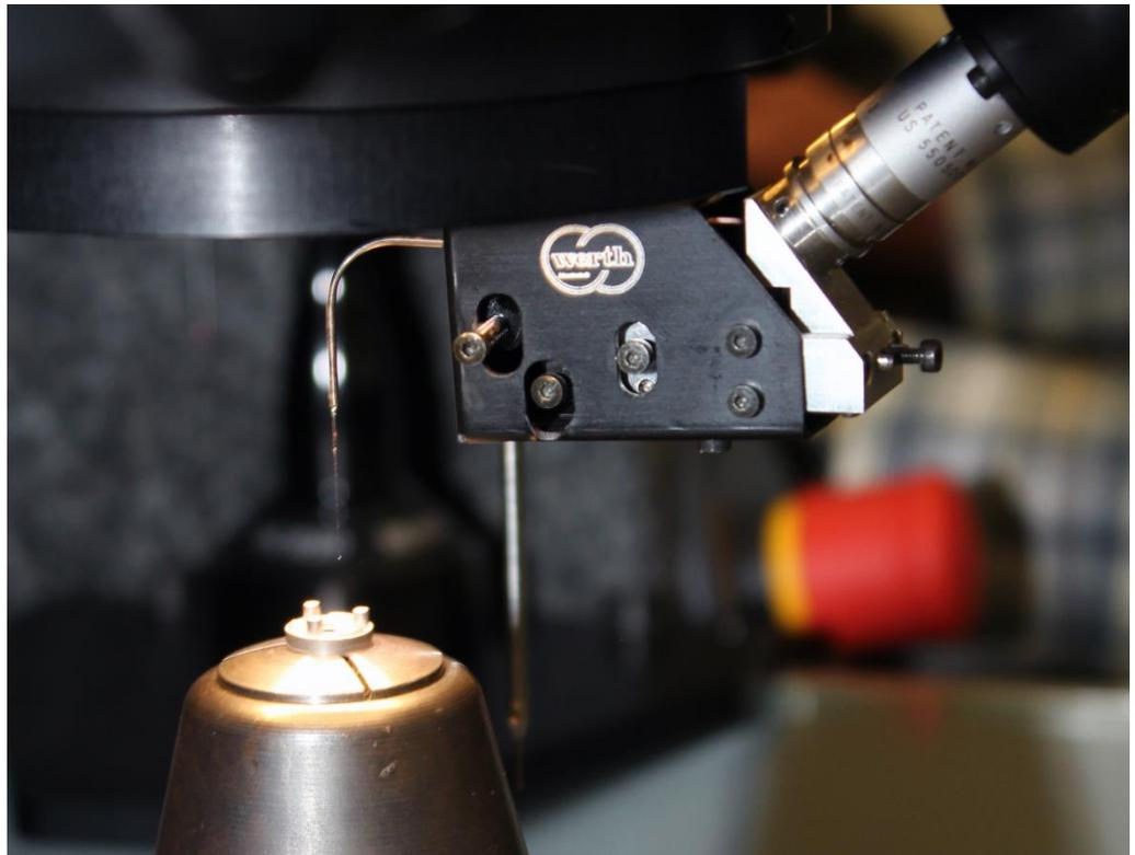
*The WFP fiber probe is a micro-probe for high-precision applications. It makes it possible to perform contacting measurements of extremely small geometries, with very small contact forces, at high precision.*
