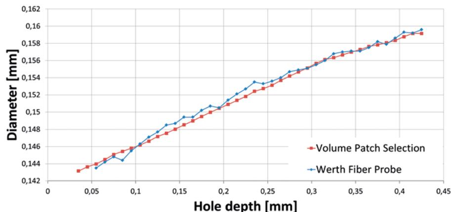
*With Volume Patch Selection, the diameter of the spray hole can be measured precisely during the entire progress, as you can see from the comparison to the Werth Fiber Probe®.*
