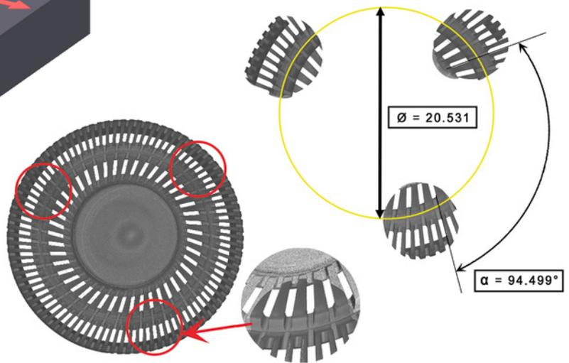
Figure 8: Using Multi-ROI CT, only the regions of interest are measured at high resolution, reducing measurement time and data volume.
