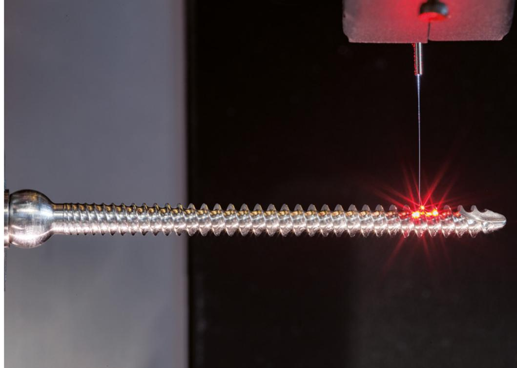
*Measuring with the Werth Fiber Probe® (WFP) a thread on a pedicle screw for stabilizing vertebral bodies*
