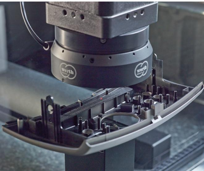
Figure 4: The patented Werth Laser Probe is integrated in the beam path of the Werth Zoom image processing sensor.
