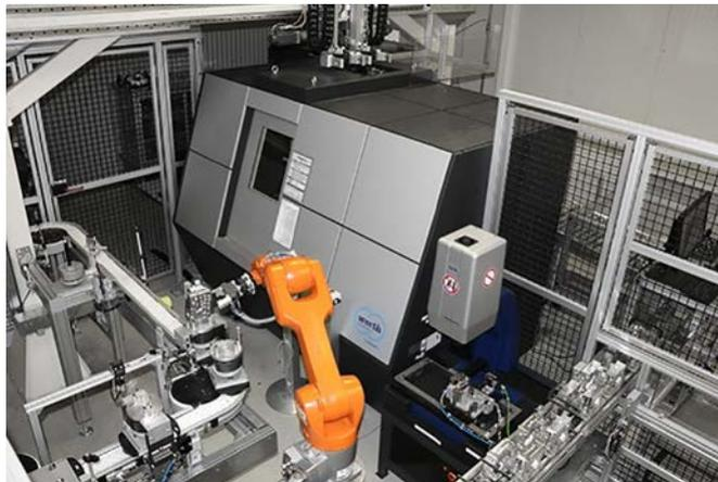
In this inline measuring cell at Continental aluminum workpieces are measured and inspected for defects in the production cycle with a TomoScope® L and a ScopeCheck® S ([werth.de/AR\\_Continental](http://werth.de/AR_Continental)).
