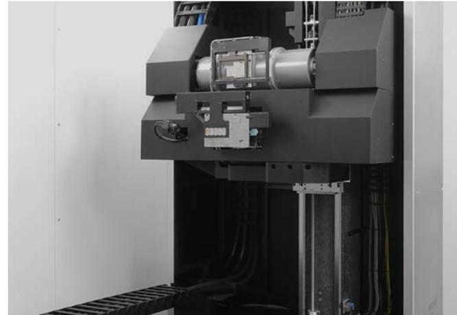
High resolution microfocus X-ray tube (down) and high power macrofocus X-ray tube (above)
