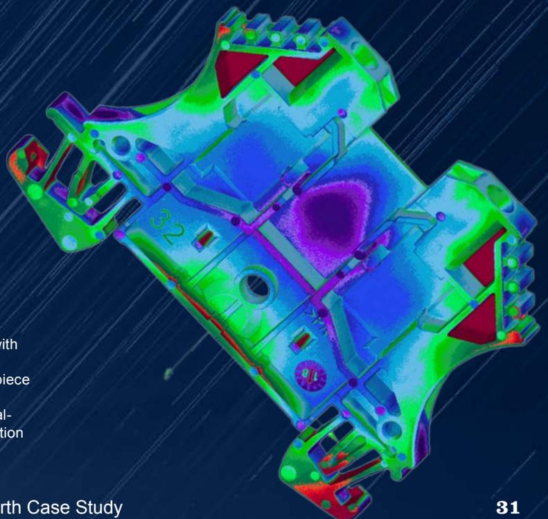
Modern Coordinate measuring machines with computed tomography sensor technology provide a complete digital twin of the workpiece in a short time. This is suitable both for dimensional measurements and for nominal-actual comparisons with color-coded deviation display. Picture: Weidmüller
