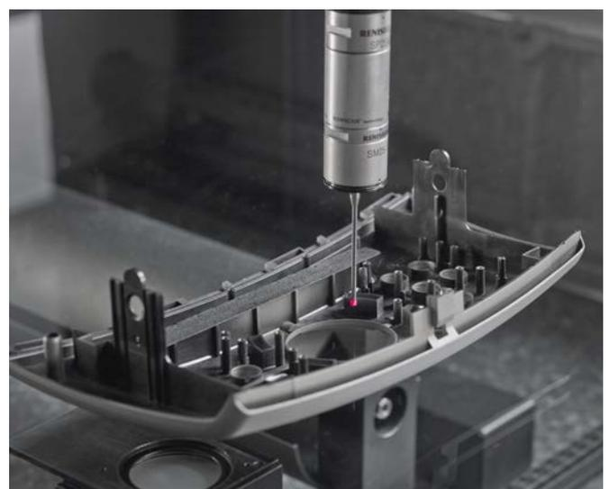
Fast alignment of the workpiece and 3D-contour measurement using the image processing system and the patented Werth Zoom with integrated Werth Laser Probe (above).
