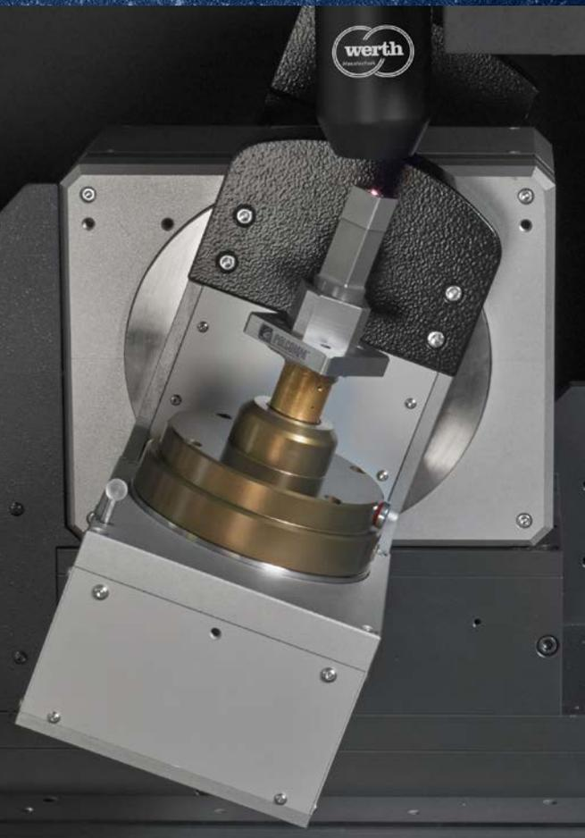
With the help of the rotary-tilt axis, surfaces that are differently oriented can be optimally aligned to the Chromatic Focus Line Sensor and then measured in workpiece coordinates.
