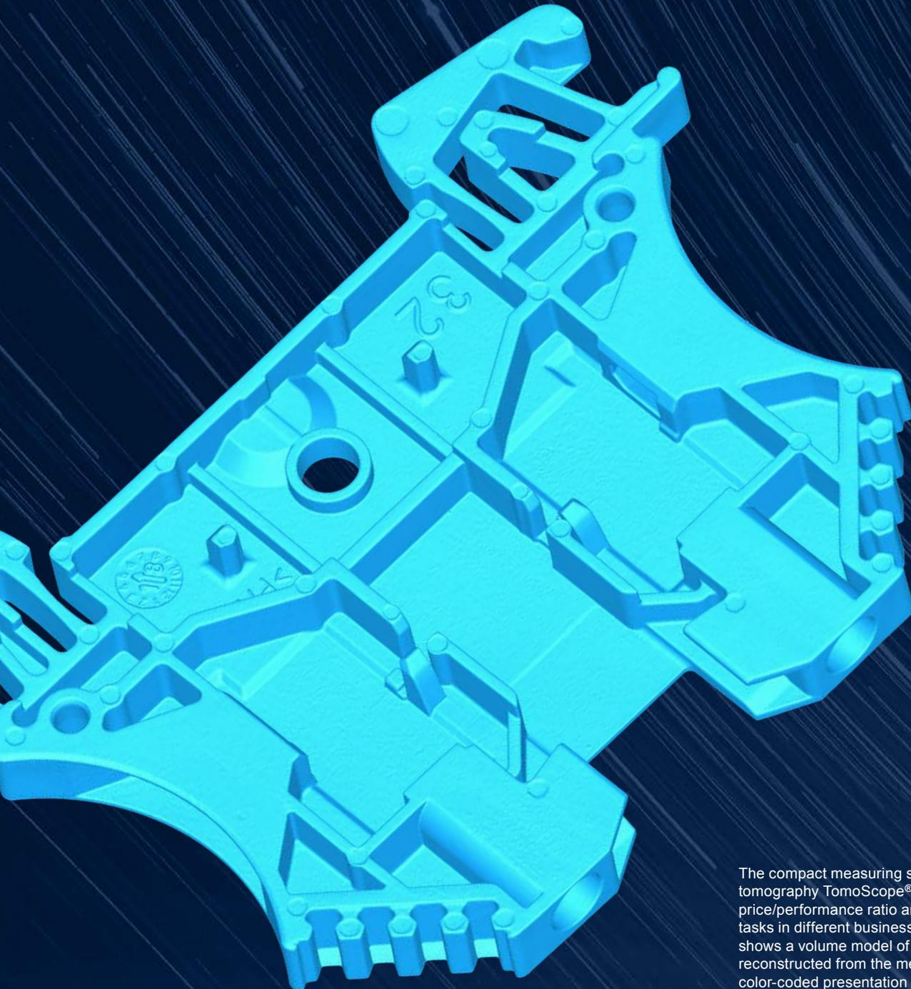
The compact measuring system with computed tomography TomoScope® XS offers a good price/performance ratio and is used for various tasks in different business areas. The picture shows a volume model of the workpiece, reconstructed from the measuring data and a color-coded presentation of the deviation from the CAD model (above).
