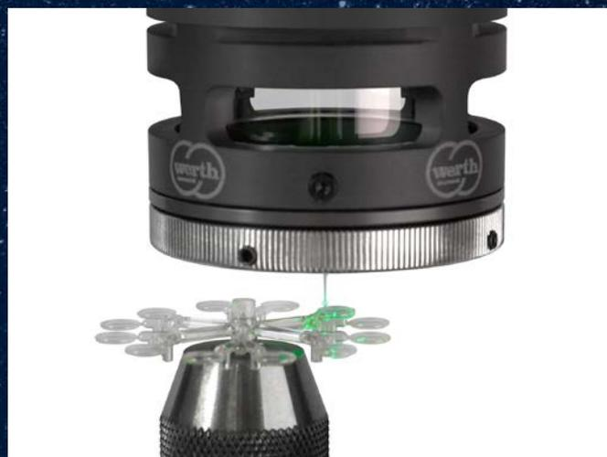
With the WFP® 3D, all parameters of the plastic lenses, including the entire surface geometry, can be measured in a single measuring sequence with manufacturing tolerances down to the sub-micron range. Mainly, the complex forms of the aspherical surfaces and their concentricity are measured. As with the LED lenses, the mounting position of plastic assemblies can also be captured using CT. Thus, the distances between the lenses, gap dimensions, and coaxiality can be measured.
