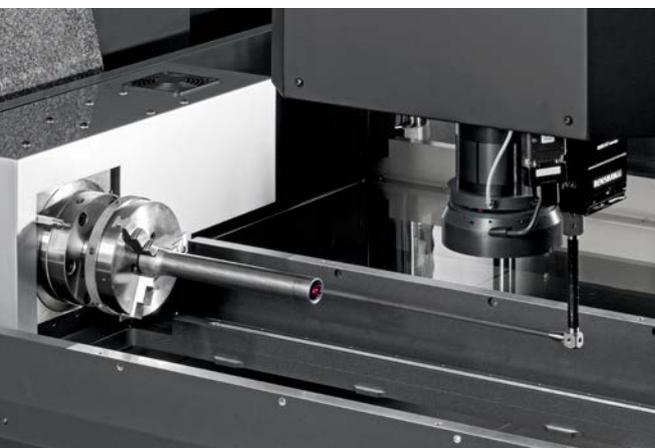
Measurements of inner contour and pitch deviations with conventional rotary axis and wobble correction by WinWerth®
