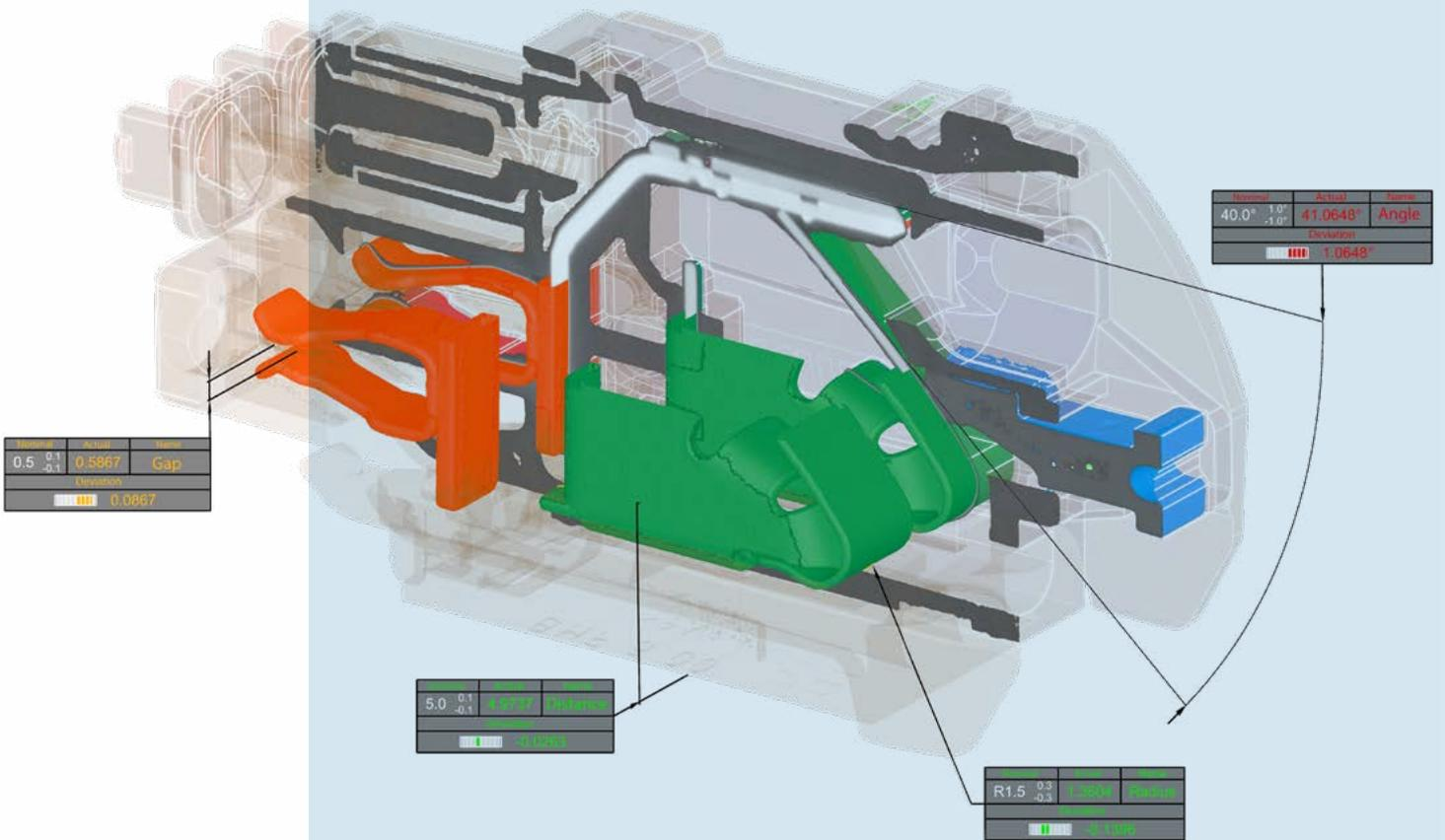
Cover picture: WinWerth® MultiMaterialScan with automatic calculation and separation of the point clouds for different plastics and metals, volume section with the different gray values of the materials as well as measured geometric properties in the WinWerth® measuring software
