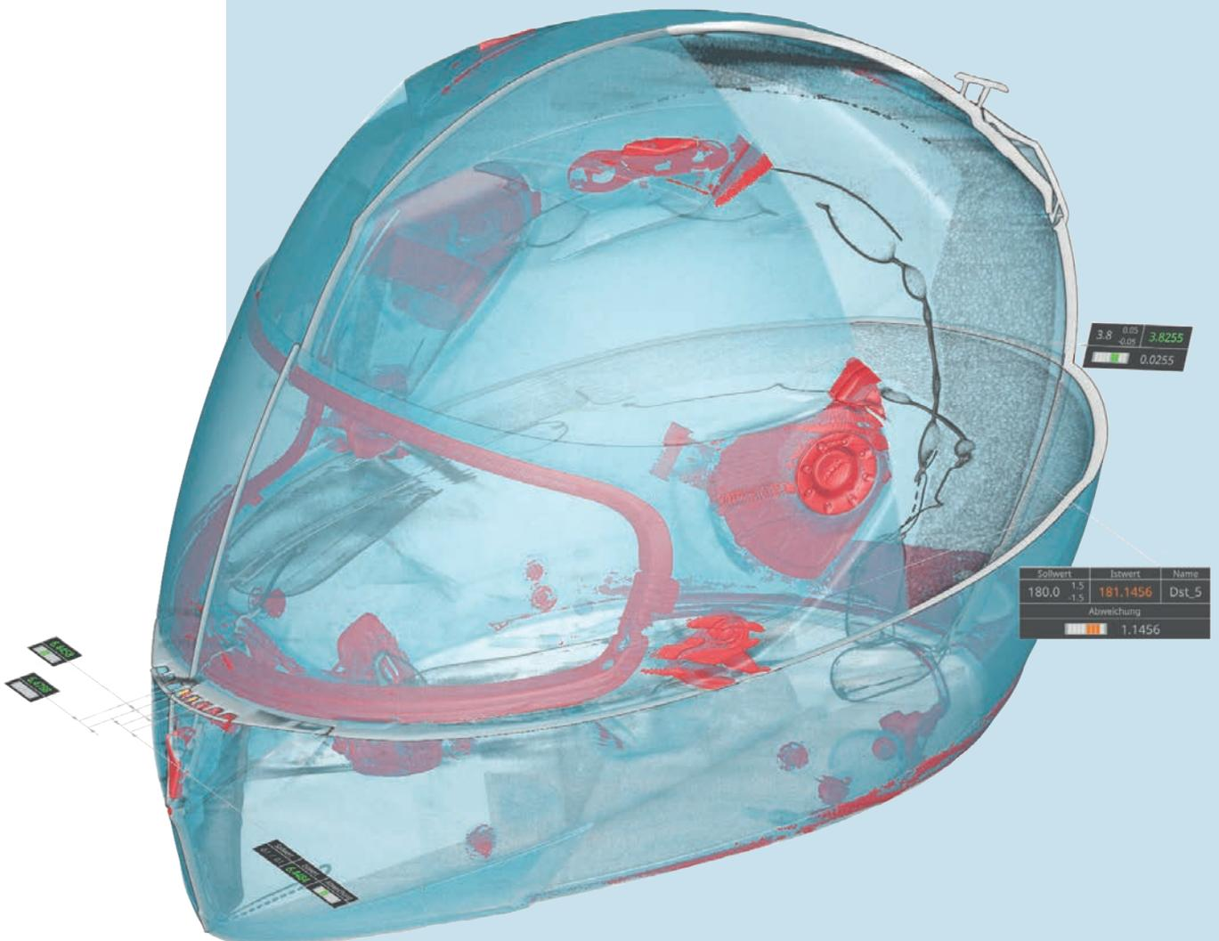
Cover picture: With the new TomoScope® S Plus and WinWerth® version 9.45, even large multi-material workpieces can be measured with the highest accuracy in this machine class
