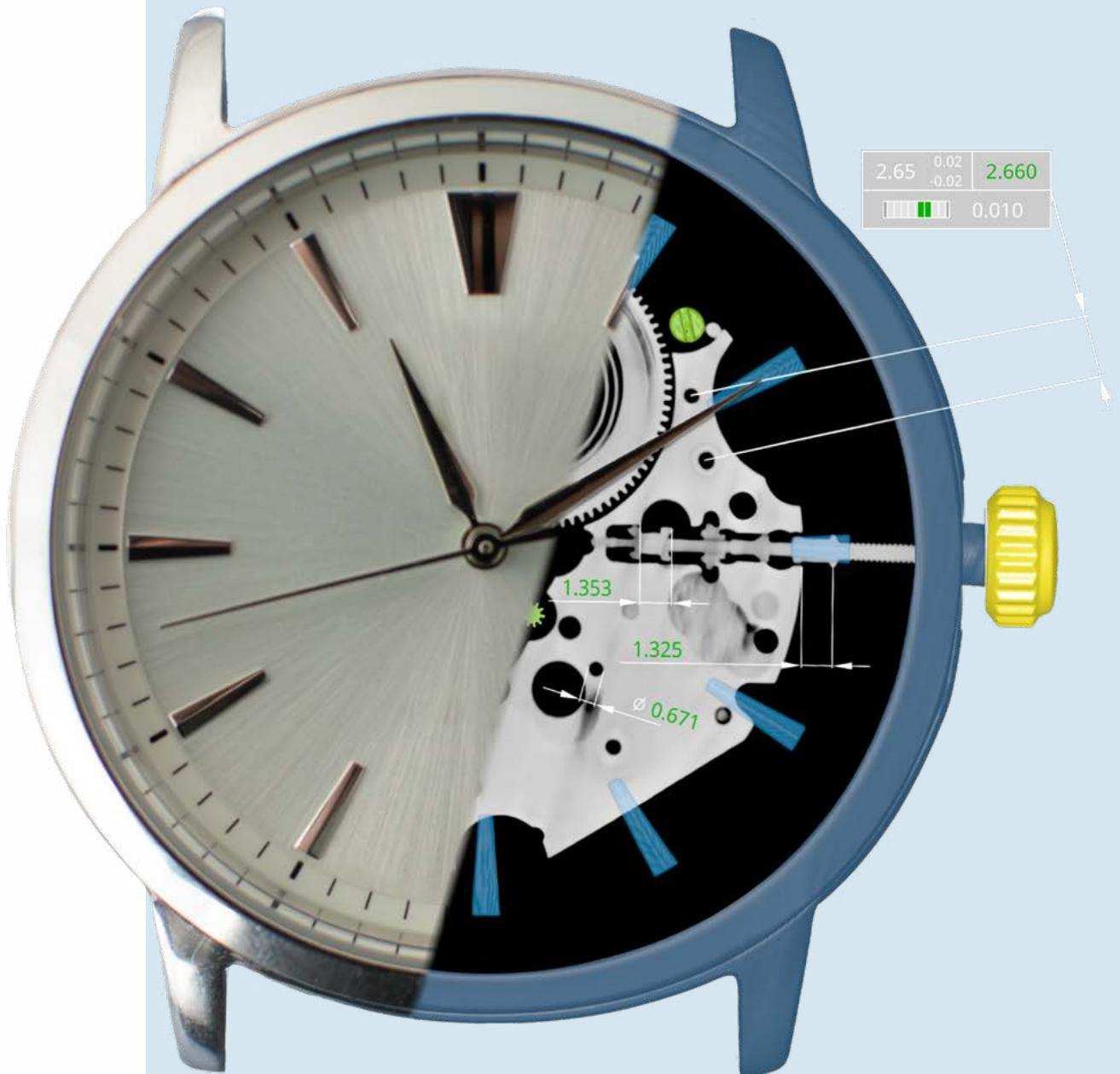
Cover image: Tomography scan of a watch mechanism with a structural resolution of a few micrometers
