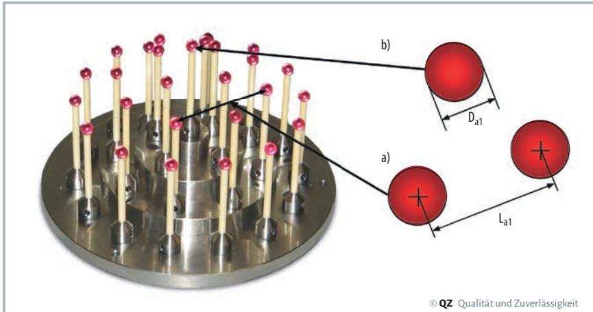
Figure 2. When length measurement error is determined from sphere center spacing, many systematic measurement errors are suppressed (a), so the error of a two-point diameter in the corresponding measurement direction between the sphere centers is added (b) (© Werth)
