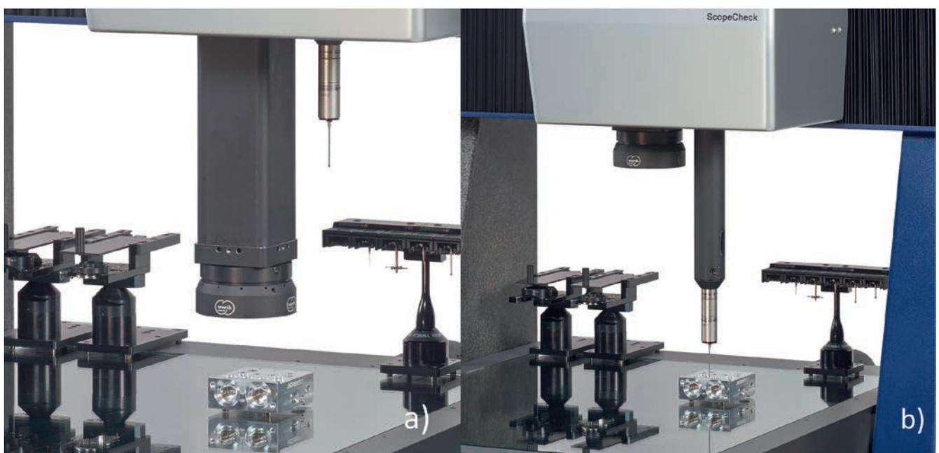
Figure 1. Programming from a CAD data set for ergonomic multisensor measurement. Application example: combined measurement using image processing (a) and tactile probe (b) (© Werth Messtechnik)
