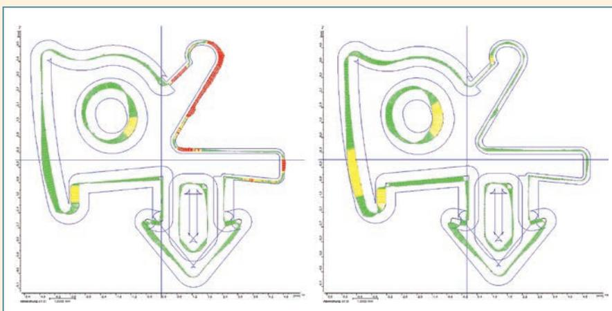
Fig. 2. When adapting the measured contour to the target contour using BestFit, the workpiece appears to be non-functional (left)—adapting using ToleranceFit, in contrast, considers the interactions between the tolerances (right)
