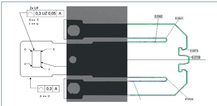
**Figure 2.** Left: drawing with line profile tolerances; center: automatic capture of the entire workpiece at high resolution with raster scanning; right: adjustment into the tolerance zones using ToleranceFit
