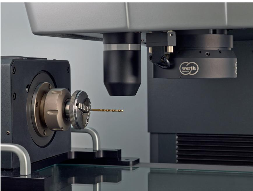
**Figure 1.** Multisensor systems on the coordinate measuring machine: Chromatic Focus Line sensor (left) and image processing sensor with integrated laser distance sensor (© Werth)
