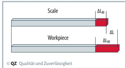
**Figure 1:** The expansions of the scale and the workpiece cancel each other out partially.
