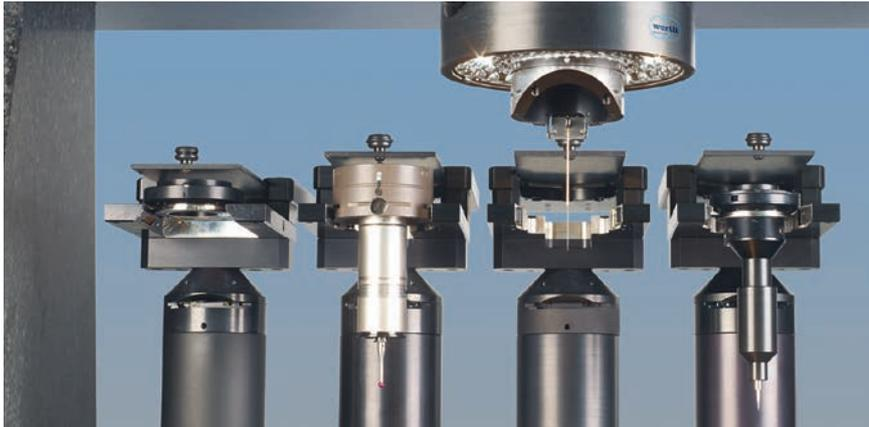
Figure 2. Using the Werth multisensor system, for example, an auxiliary lens for the integrated laser distance sensor, conventional probe systems, fiber probes, and contact stylus sensors can be changed out with zero offset in front of the beam path of the image processing sensor. (© Werth)
