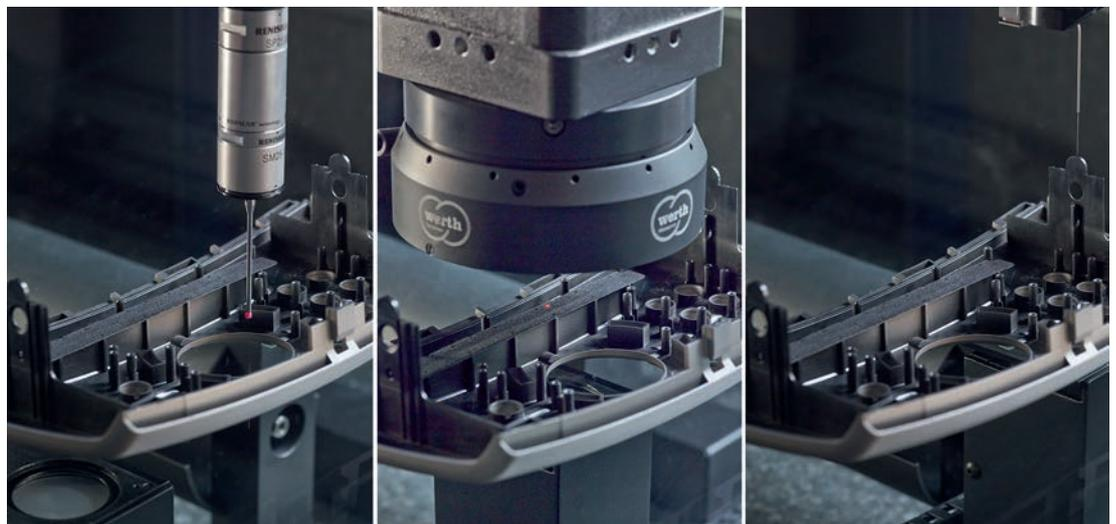
Figure 1. Tactile (left), optical (center), and tactile-optical (right) multisensor systems
